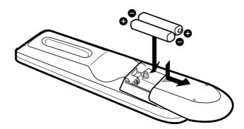
Slide the cover on the back of the remote down towards the bottom of the remote control. Insert two batteries carefully noting the "+" and "-" markings, placing the "-" end in the unit first. Slide the cover back into place.
